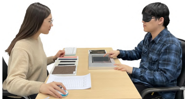
Fig. 8. The experimental setup. The participant sits at one side of the table and explores the virtual textures; meanwhile, the experimenter sits at the other side of the table to transpose the real material samples and records the participant’s response.
