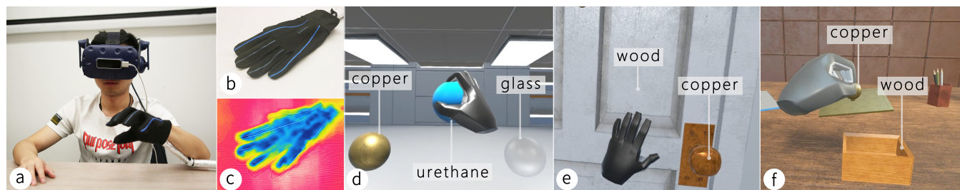
Figure 1: (a) a user wearing ThermAirGlove ( TAGlove ) and grasping the virtual object in VR, (b) the RGB image of TAGlove , (c) the thermal image of TAGlove filled with cold air, (d-f) Examples of TAGlove applications in virtual scenes, left to right: three virtual spheres with different materials, a wood door with a copper handle, a wood box with a copper lid.
